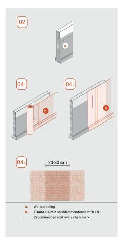
In drainage applications T-Kone G Drain is used with the geotextile facing towards the backfill, i.e. the flat side on the wall.
